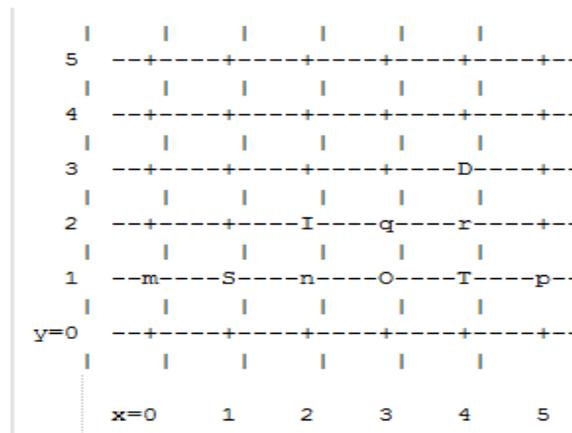
In a pristine fabric, torus-2QoS would generate the path from S to D as S-n-O-T-r-D. With failed switches O and T, torus-2QoS will generate the path S-n-I-q-r-D, with illegal turn at switch I, and with hop I-q using a VL with bit 1 set. In contrast to the earlier examples, the second hop after the illegal turn, q-r, can be used to construct a credit loop encircling the failed switches.
